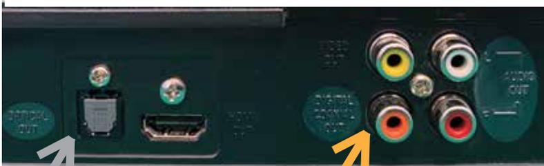
If there is a **DIGITAL COAXIAL (COAX)** or **OPTICAL OUT**, the optional **DIGITAL inLOOP CONNECTOR** will connect digital outputs to LC inLOOP (see instructions on HOME inLOOP).
