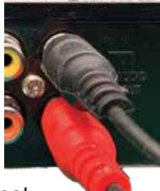
There are a number of different types of audio outputs. If your system has a left (L) and right (R) AUDIO OUT like the photo to the left, install the included cable from this output to the "Line" input on LC inLOOP, like the photos below.
